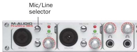
Mic/Line selector on the front of a FireWire 1814
